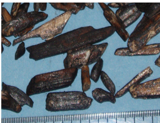
Figure 2. Oversized wood particles recovered from the ash bath after passing through a power plant boiler.
